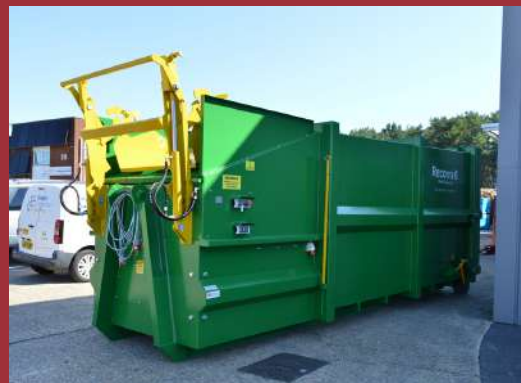
MC32BL Mobile Compactor with Bin Lift with added Greedy Boards for a site with a lot of crosswinds.
