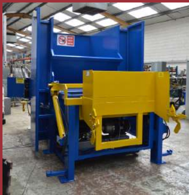
SC3000BL Rear Ground Bin Lift, not a common set up but works perfect in the right situations.
