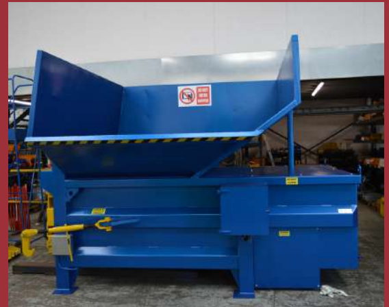
Refurbished Static Compactor designed for emptying bins with a fork lift
