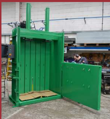
HB550 Mill Size Baler with the bottom door hinged the opposite way from standard.
