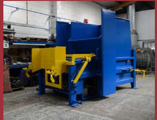
SC3000BL Rear Ground Bin Lift, not a common set up but works perfect in the right situations.
