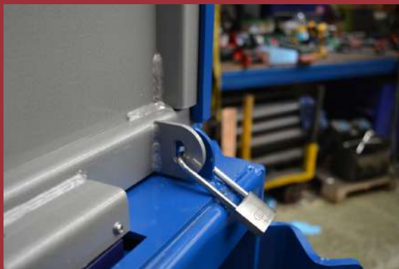
HB550 Mill Size Baler with an additional Padlock shackle on the top door to prevent unauthorised use.
