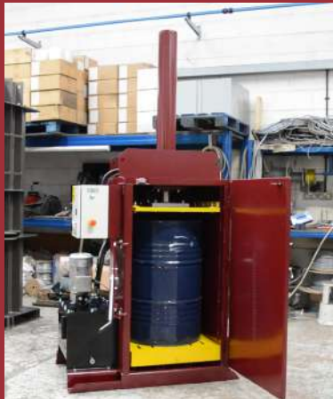
DC205 Drum Crusher with a fast cycle module upgrade. As this one was for a site further North Guy Saunders installed this one.
