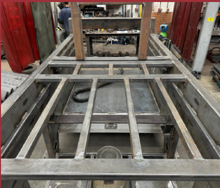
Reinforcements on the frame
