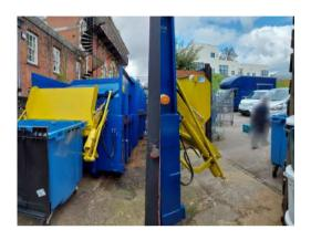
We refurbished a 32yd mobile compactor for a trade partner, but this wasn't just a standard refurb project; we replaced the powerpack with one of ours found in the MC32 model so they could have SmarTec
